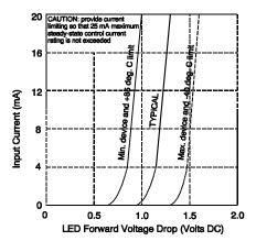
Figure 5. Input Characteristics (Current Controlled)
