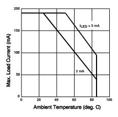
Figure 1. Typical Current Derating Curve
