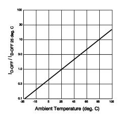
Figure 4. Typical Normalized Off-State Leakage
