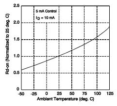
Figure 3. Typical Normalized On-Resistance
