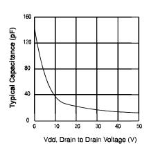
Figure 8. Typical Output Capacitance
